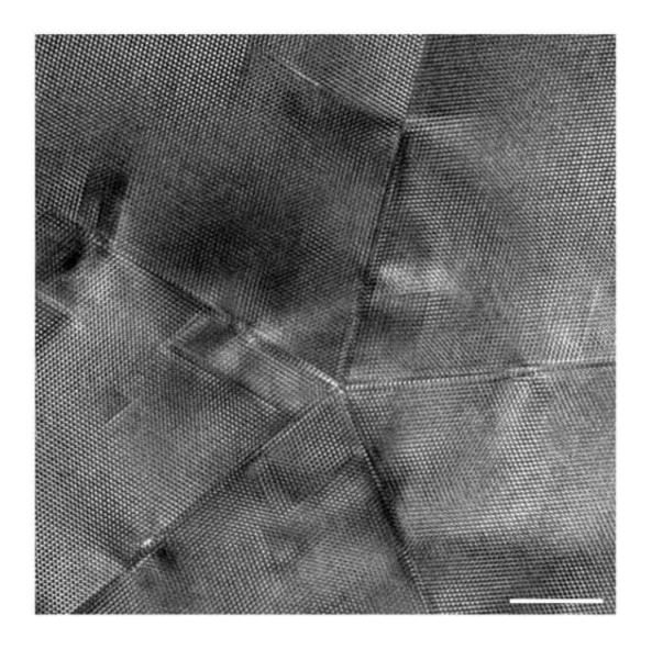
A high-resolution transmission electron microscopy image of the core of a single silver nanowire. The scale bar represents 5 nm in length. The image was taken on the Argonne Chromatic Aberration-corrected TEM (ACAT) machine. Image: Argonne National Laboratory
