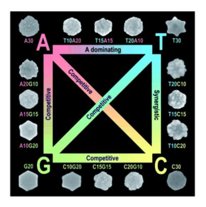
Gold nanoparticles are made by sewing tiny gold seeds in a solution of gold salt. Particles grow as gold in the salt solution deposits onto the seeds. Lu's group incubated the gold seeds with short segments of DNA before adding the salt solution, causing the particles to grow into various shapes determined by the genetic code of the DNA.
