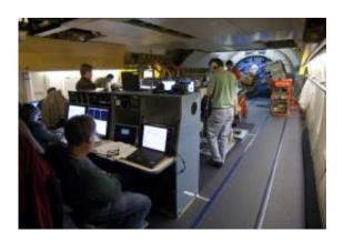
Astronomers and mission operations staff monitor data at their consoles during a science flight aboard the SOFIA flying observatory. The FORCAST instrument is mounted on the blue pressure bulkhead; the telescope itself is mounted on the other side of the bulkhead. (NASA/DLR/USRA/DSI/FORCAST team)
