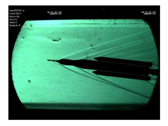
The 70-metric-ton configuration of the SLS rocket, designed to carry the Orion spacecraft, is tested in the Trisonic Wind Tunnel at NASA's Marshall Space Flight Center. This view uses special cameras and a deflection of light directed through the windows in the tunnel to show the shadows of airflow as it changes angles at high speeds, helping visualize the various intense pressures of atmosphere on the model. Credit: NASA/MSFC
