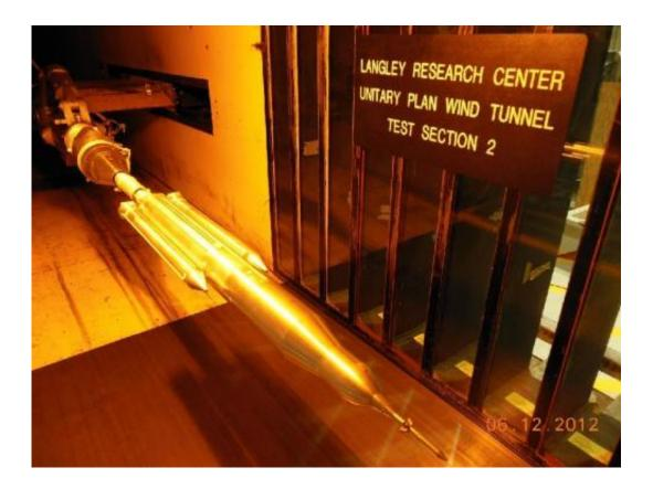
Wind tunnel testing on the 70-metric-ton configuration of SLS, conducted at the Langley Research Center. Credit: NASA/LaRC
