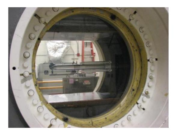
Engineers at the Marshall Center test the 130-metric-ton heavy-lift configuration of the Space Launch System rocket in the Trisonic Wind Tunnel in Bldg. 4732. Credit:NASA/MSFC
