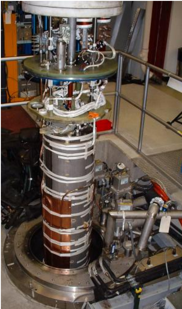
An 11 T magnet ready for cryogenic testing.
