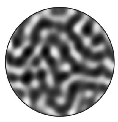
An image of a nanoscale ferromagnetic structure made using a new single-shot X-ray holography technique perfected at the Soft X-ray Materials Science instrument at SLAC's Linac Coherent Light. Image: Tianhan Wang
