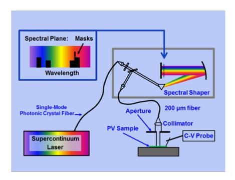
Diagram of Lab apparatus. The laser output is sent to a prism which splits the light into its constitutent wavelengths. Masks are inserted into the prism beam to shape the spectrum. The result is routed to a collimator and focused onto PV samples.
