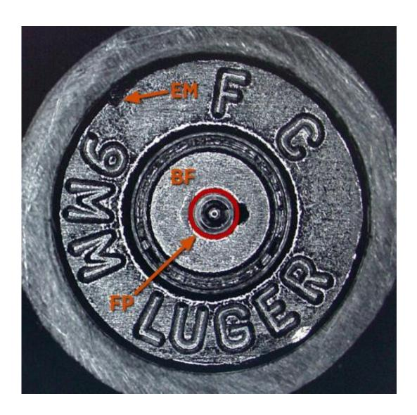
This cartridge case shows the three distinct marks, or 'signatures,' impressed on its surface when it was fired by a gun: the firing pin impression (FP), the breech face impression (BF) and the ejector mark (EM). NIST's standard casing ensures that forensic labs can accurately match signatures on shells found at crime scenes
