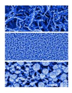
These color-enhanced scanning electron microscope images show nanosheets resembling tiny rose petals. The nanosheets are key components of a new type of biosensor that can detect minute concentrations of glucose in saliva, tears and urine. The technology might eventually help to eliminate or reduce the frequency of using pinpricks for diabetes testing. (Purdue University photo/Jeff Goecker)
