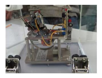
VBB seismometers, such as this prototype, are tested at the Black Forest Observatory for use on the moon and mars. Photo: Rudolf Widmer-Schnidrig
