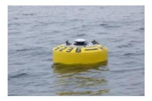
A new network including data receivers on Wave Gliders and fixed buoys will pick up signals from acoustic tags on animals passing within 1,000 feet and transmit the data to a research team on shore, led by Stanford University Marine Sciences Professor Barbara Block. Credit: Kip Evans
