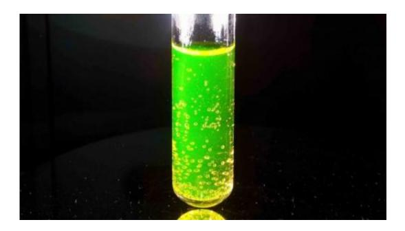
(Phys.org)—Scientists at the University of Cambridge have produced hydrogen, H<sub>2</sub>, a renewable energy source, from water using an inexpensive catalyst under industrially relevant conditions (using pH neutral water, surrounded by atmospheric oxygen, O<sub>2</sub>, and at room temperature).
