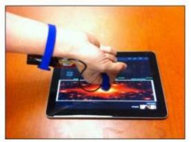
The prototype ring and its usage for transmitting short messages from the ring to a touchpad. Image credit: Tam Vu
