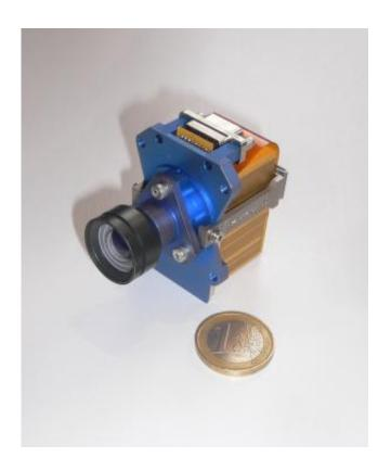
Proba-2's wide-viewing Exploration Camera (X-Cam) is one of 17 new technologies being tested by this small satellite. The X-Cam, produced by Swiss company Micro-Cameras & Space Exploration, is only about the size of an espresso cup but can produce 100° field of view monochrome images. Credits: ESA/Micro-Cameras & Space Exploration
