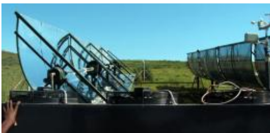
The Solar ORC setup in Lesotho. Photo: STG International
