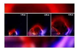
Plasma loops created in the lab were recorded using high-speed cameras. Credit: Eve Stenson / California Institute of Technology
