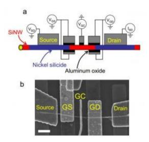
a) Schematic of a multi-gate device made from a single, undoped SiNW. Two wrap-gates, labeled as GS and GD, are designed to control the Schottky barriers at the silicidesilicon junctions formed by the source and drain contacts. The finger gate in the middle, labeled as GC, is meant to control carrier population in the silicon channel. b) SEM micrograph of the device. Scale bar: 400nm. Image: arXiv:1208.1465v1
