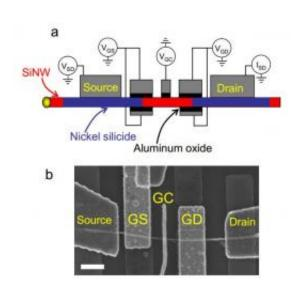
a) Schematic of a multi-gate device made from a single, undoped SiNW. Two wrap-gates, labeled as GS and GD, are designed to control the Schottky barriers at the silicidesilicon junctions formed by the source and drain contacts. The finger gate in the middle, labeled as GC, is meant to control carrier population in the silicon channel. b) SEM micrograph of the device. Scale bar: 400nm. Image: arXiv:1208.1465v1
