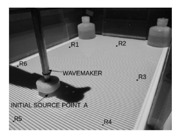
In the water tank, Point A is the original source of the wave, while the surrounding R points correspond to positions where the wave is measured and reemitted after the time reversal operation. Image credit: A. Przadka, et al. ©2012 American Physical Society
