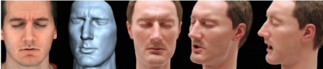
Left: photograph and scanned 3D geometry of a human face. We use a physics-based optimization process to design the geometry of a synthetic skin in order to best match given target expressions. Right: final animatronic figure with fabricated skin.
