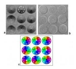
MTXM images of in-plane (a) and out-of-plane (b) magnetic components in an array of permalloy nanodisks. In-plane magnetic rotation is shown by white arrow (a). Core polarization is marked by black (up) and white (down) spots. Image (c) shows the complete vortex configuration of each nanodisk in the array. (Images courtesy of Im and Fischer)
