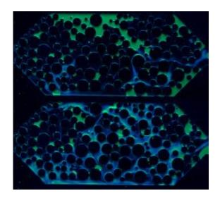
As biofilm, represented in blue, grows in this micromodel, it clogs up some pore spaces. This allows recovery of more oil, seen in the lower image as less of the green color. (Graphic courtesy of Oregon State University)
