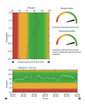
A speedometer-type reading of fish welfare makes it simple to monitor environmental conditions in the cage. Screenshot: www.imr.no/welfaremeter
