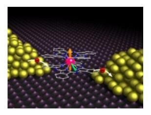
This is the TbPc2 molecule quantum-bit device. Electrons (red) from the electrodes jump onto the molecule reading out the electronic spin (orange) and the nuclear spin (green). Credit: Graphics: C. Grupe, KIT
