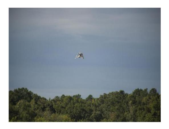
The "Mighty Eagle" soars above the tree line. The vehicle was "open loop"--navigating autonomously without the command of the onboard camera
