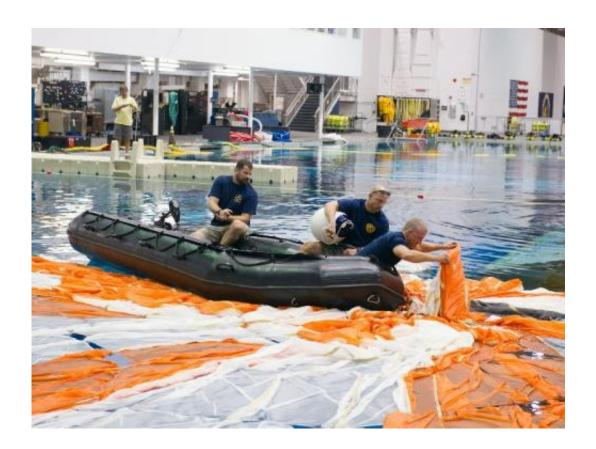
Personnel from NASA's Johnson Space Center and Kennedy Space Center practice recovering Orion's parachutes at the Neutral Buoyancy Laboratory in Houston. The teams were determining the best methods for retrieving the chutes from the water after Orion's splashdown. Each main chute weighs close to 300 pounds, and the water doubles that weight. Photo credit: NASA
