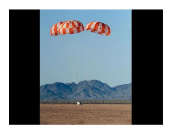
A C-17 plane dropped a test version of Orion from an altitude of 25,000 feet above the U.S. Army Yuma Proving Ground in southwestern Arizona. This test was the second to use an Orion craft that mimics the full size and shape of the spacecraft. The main objective of the latest drop test was to determine how the entire system would respond if one of the three main parachutes inflated too quickly. Photo credit: NASA
