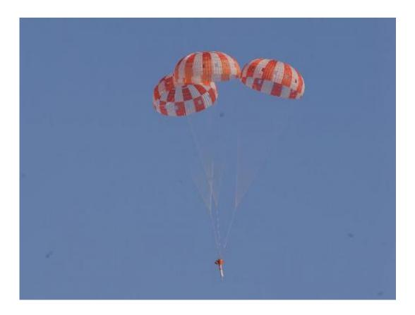
A dart-shaped test vehicle that is used to simulate Orion's parachute compartment descends above the skies of the U.S. Yuma Army Proving Ground in Arizona. Engineers were testing the maximum pressure Orion's chutes might face when returning from exploration missions. Photo credit: NASA
