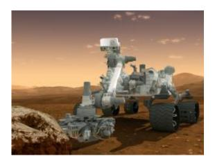
This artist's concept features NASA's Mars Science Laboratory Curiosity rover, a mobile robot for investigating Mars' past or present ability to sustain microbial life. Image credit: NASA/JPL-Caltech
