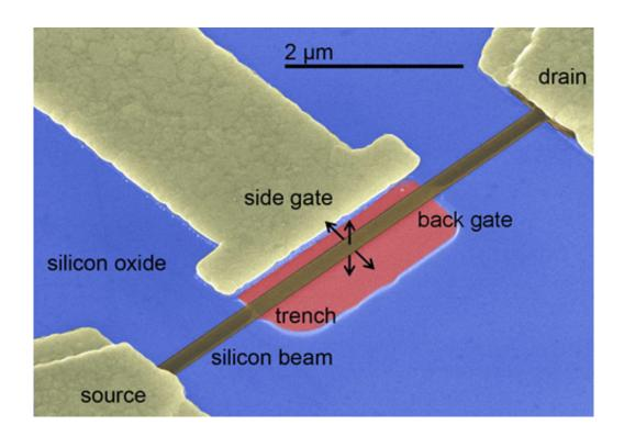
This image from a scanning electron microscope shows a tiny mechanical device, an electrostatically actuated nanoresonator, that might ease congestion over the airwaves to improve the performance of cell phones and other portable devices. (Purdue University image)
