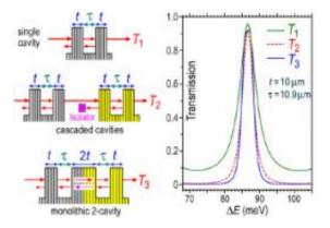
Fabry-Perot resonance spectra (right) of a single-cavity resonator, two cascaded resonators, and a monolithic two-cavity resonator, respectively. Note the significant background of T1 as the Bragg reflectivity from a 10-µm diamond plate is only 59%. By comparison, spectra T2 and T3 are very similar, both having sharp tails and extremely low background. Diamond 224 back reflection (E = 8.5146 keV, Dawin range  $67 \le \Delta E \le 106$  meV).
