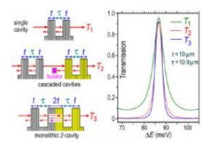
Fabry-Perot resonance spectra (right) of a single-cavity resonator, two cascaded resonators, and a monolithic two-cavity resonator, respectively. Note the significant background of T1 as the Bragg reflectivity from a 10- $\mu$ m diamond plate is only 59%. By comparison, spectra T2 and T3 are very similar, both having sharp tails and extremely low background. Diamond 224 back reflection (E = 8.5146 keV, Dawin range 67  $\leq \Delta E \leq 106$  meV).
