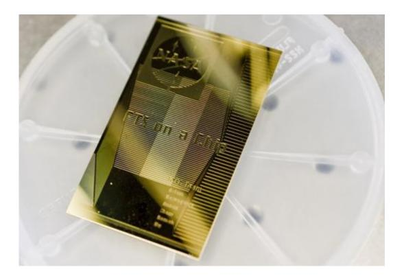
This is a close-up view of the "spectrometer-on-a-chip" technology that could dramatically reduce the size of spectrometers in the future. (Credit: NASA Goddard/Chris Gunn)
