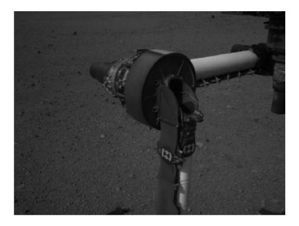
This full-resolution image from NASA's Curiosity shows the elbow joint of the rover's extended robotic arm on Aug. 20, 2012. The Navigation Camera captured this view. Image credit: NASA/JPL-Caltech
