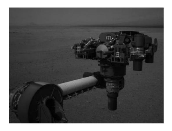
This full-resolution image from NASA's Curiosity shows the turret of tools at the end of the rover's extended robotic arm on Aug. 20, 2012. The Navigation Camera captured this view. Image credit: NASA/JPL-Caltech
