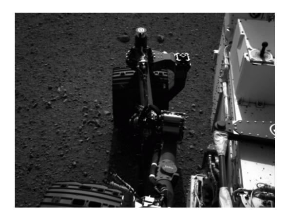
(CLICK ENLARGE) This set of images shows the movement of the rear right wheel of NASA's Curiosity as rover drivers turned the wheels in place at the landing site on Mars. Engineers wiggled the wheels as a test of the rover's steering and anticipate embarking on Curiosity's first drive in the next couple of days. This image was taken by one of Curiosity's Navigation cameras on Aug. 21. Image credit: NASA/JPL-Caltech
