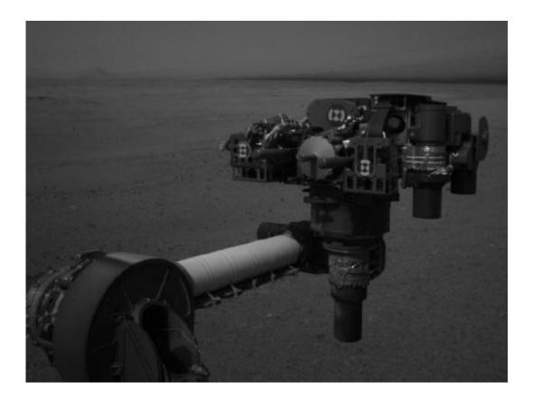
This full-resolution image from NASA's Curiosity shows the turret of tools at the end of the rover's extended robotic arm on Aug. 20, 2012. The Navigation Camera captured this view. Image credit: NASA/JPL-Caltech
