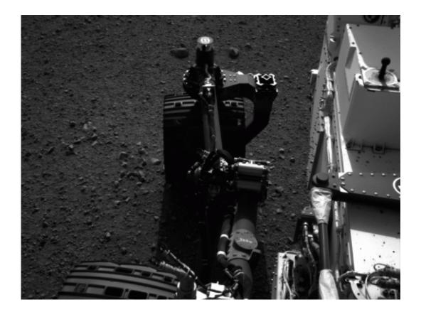
(CLICK ENLARGE) This set of images shows the movement of the rear right wheel of NASA's Curiosity as rover drivers turned the wheels in place at the landing site on Mars. Engineers wiggled the wheels as a test of the rover's steering and anticipate embarking on Curiosity's first drive in the next couple of days. This image was taken by one of Curiosity's Navigation cameras on Aug. 21. Image credit: NASA/JPL-Caltech
