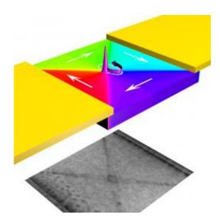
The color graphic above a transmission electron microscope image of the vortex core shows the trapped spins moving around the permalloy sample, which then generate the conical vortex core rising out of the center.
