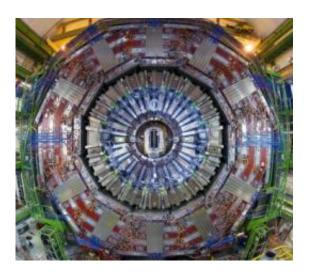
A view of the detector in the 12,500-ton Compact Muon Solenoid experiment (CMS). Image courtesy of CERN
