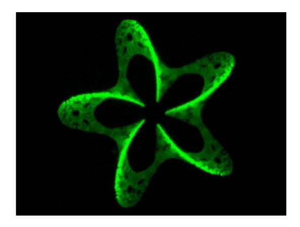
3D pattern, produced by photografting (180 µm wide). Fluorescent molecules are attached to the hydrogel, resulting in a microscopic 3D pattern.
