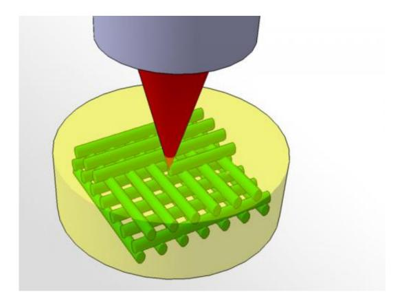
3D Photografting: A laser shines into the hydrogel (yellow), attaching molecules to it at specific points in space (green).
