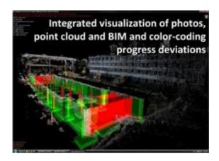
This image shows the integrated visualization of photos taken at the construction site, and the color coding allows someone monitoring the progress to understand where performance deviations may be occurring. Credit: Virginia Tech
