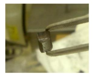
A freshly cast research sample of delta plutonium.
