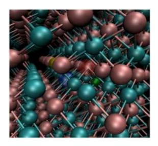
Atomic structure of co-dopant complex in thallium bromide that binds charged vacancies and reduces their mobility, allowing selective control over ionic conductivity without affecting electronic conductivity.
