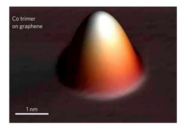
This zoom-in STM topograph shows one of the cobalt trimers placed on graphene for the creation of Coulomb potentials - charged impurities - to which electrons and holes could respond. (Image courtesy of Crommie group)
