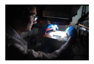
IBM increases world record to 11.1 percent for a high-efficiency solar cell made from earth-abundant materials. IBM Researcher Teodor Todorov (pictured) tests a solar cell made of Cu2ZnSn(S,Se)4 (readily available copper, zinc, and tin, and referred to as CZTS) in a solar simulator equal to the power of one sun. This breakthrough holds potential for solar cell technology to produce more energy at a lower cost and with less barriers to scale.
