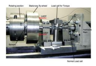
Researchers used a rotary shear apparatus to identify 'melt welts.'
