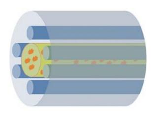
Processing biological samples on a small substrate the size of a computer chip is becoming a common task for biotechnology applications. Given the small working area, however, probing samples on the substrate with light can be difficult. To address this issue, Xia Yu and co-workers at the A\*STAR Singapore Institute of Manufacturing Technology have now developed an optical fiber system that is able to deliver light to microfluidic chips with high efficiency.
