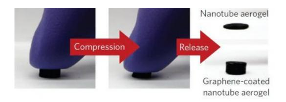
After CNT aerogels are compressed and released, the non-coated aerogel collapses while the graphene-coated aerogel recovers its original shape. Image credit: Kim, et al. ©2012 Macmillan Publishers Limited
