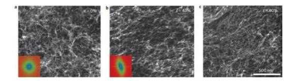
As compression increases in this sequence of images, the graphene-coated nanotubes undergo increasing alignment, strengthening the aerogel. Image credit: Kim, et al. ©2012 Macmillan Publishers Limited
