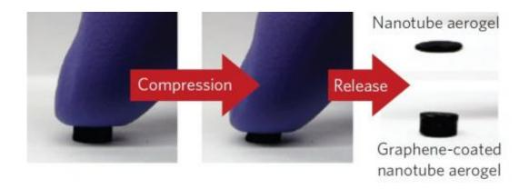
After CNT aerogels are compressed and released, the non-coated aerogel collapses while the graphene-coated aerogel recovers its original shape. Image credit: Kim, et al. ©2012 Macmillan Publishers Limited
