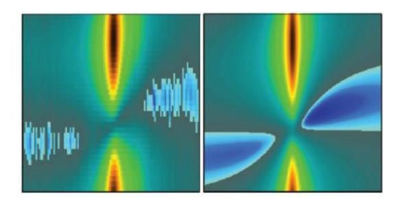
Berkeley Lab researchers directly observed quantum optical effects -- amplification and ponderomotive squeezing -- in an optomechanical system. Here the yellow/red regions show amplification, the blue regions show squeezing. On the left is the data, on the right is the theoretical prediction in the absence of noise. Credit: (Photo courtesy of Stamper-Kurn group)
