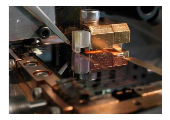
Dan Stamper-Kurn's research group has developed a microfabricated atom-chip system which provides a magnetic trap for capturing a gas made up of thousands of ultracold atoms. Credit: (Photo courtesy of Stamper-Kurn group)
