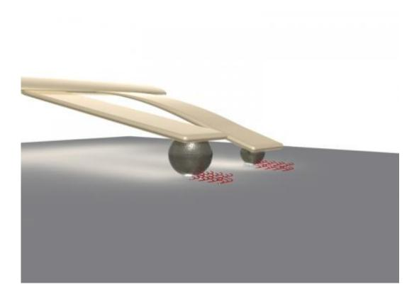
This technique uses no electronic components to bring the cantilevers into contact with the substrate surface. Credit: Albena Ivanisevic, North Carolina State University
