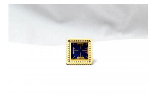
Sensor developed by Nosang Myung that can detect airborne toxins
