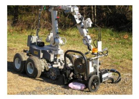
The SAPBER pipe bomb dismantler takes the pipe bomb from a bomb-disposal robot, disassembles it, empties the pipe, makes a video, and carefully preserves all of the evidence. Credit: RE2 Inc.
