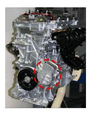
Aisin Seki electric water cooling pump installed in engine (red circle) © Aisin Seiki
