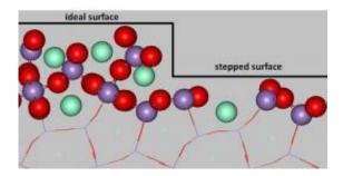
Side view of ideal and stepped crystal surface of Noxicat. Nitrogen oxide oxidation occurs preferentially on the stepped surface. Image: Geoffrey McCool
