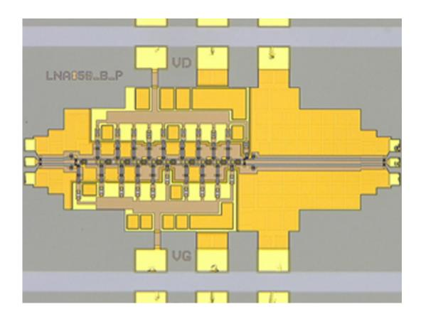
DARPA researchers have created the world's first solid state receiver to demonstrate gain at 0.85 terahertz (THz).
