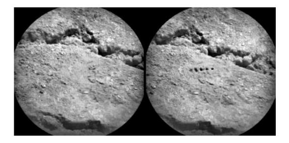
Before-and-after images from Curiosity's ChemCam micro-imager show holes left by its million-watt laser. Credit: NASA/JPL-Caltech/LANL/CNES/IRAP/LPGN/CNRS
