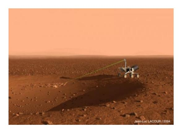
ChemCam's laser allows Curiosity to zap and examine targets up to 23 feet (7 meters) away. Credit: J-L. Lacour/CEA/French Space Agency (CNES)
