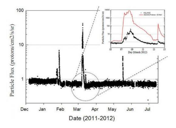
RAD charged particle flux observations during ~7 months of cruise included contributions from 5 solar energetic particle events. The inset compares the particle flux observed by RAD to that observed by instruments on the ACE spacecraft. The MSL spacecraft structure (backshell, heatshield, etc.) provided significant shielding from deep space radiation, significantly reducing the particle flux compared to ACE. Credit: NASA/ACE/RAD
